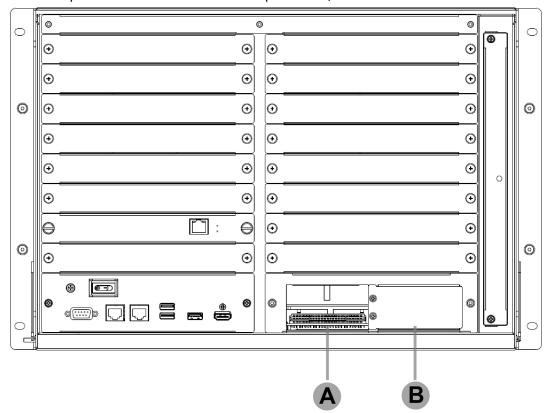
3. Slide the power module to the power slot. A click sound is made once the power module is properly installed.
