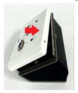
6 Secure the transmitter to the mounting plate with the four M3x8 screws provided.
