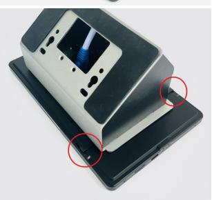
6 Secure the Touch Panel to the mounting plate with the screw you removed at step 2.
