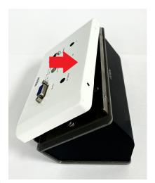
7 Secure the transmitter to the mounting plate with the four M3x8 screws provided.
