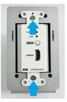
Attach the faceplate by pressing it onto the transmitter until it locks in place.
