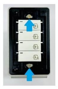
7 Attach the faceplate by pressing it onto the target device until it locks in place.
