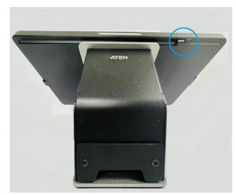
6 Secure the Touch Panel to the mounting plate with the screw you removed at step 3.
