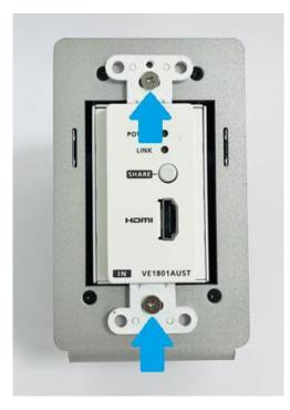
Attach the faceplate by pressing it onto the transmitter until it locks in place.
