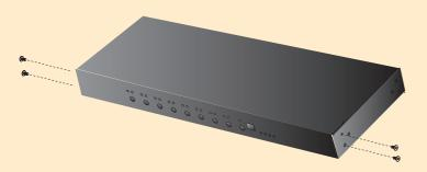
2. Screw the rack mounting brackets into the front and rear modules.
