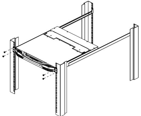
**3.** After the front brackets are secured, tighten all the screws.
