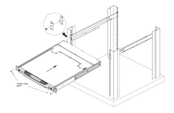
**4.** Stabilize the LCD unit further by screwing an M4\*6 Type I Screw to each of the unit's *rear attachment sliding brackets*.
