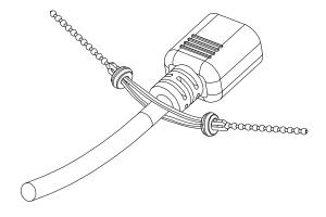
Using a Lok-u-Plug Installation Tool, lock the part of the Cable Holder inserted into the hole by pushing it towards the small part of the hole.
