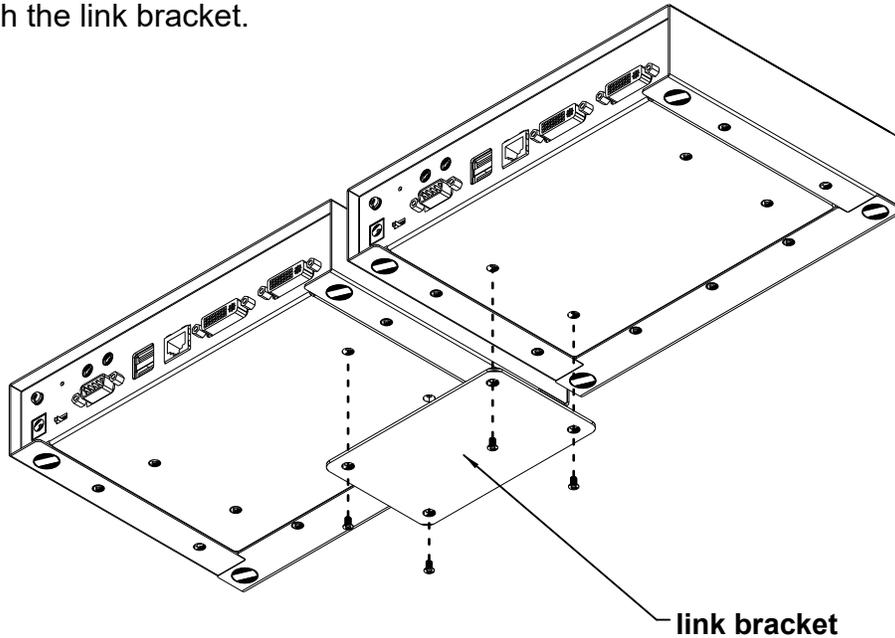
2. Remove the bottom and side screw from each KE Series unit.
