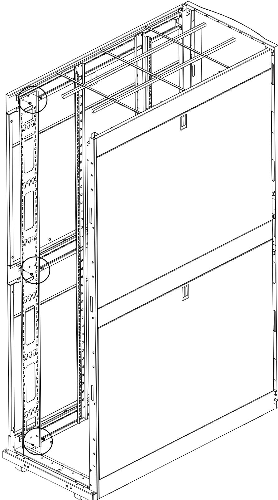
Once installed, users can mount ATEN PDUs, with their cords at the bottom / top of the Mount Rail, by sliding them into place.
