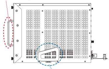
To transport the unit, use the recessed handles, but not the 2 front handles.
