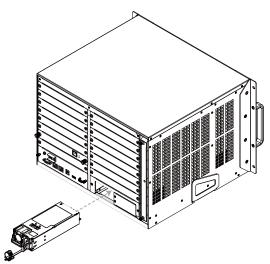
4. Plug the power cord into the 3 prong socket of the power module.
