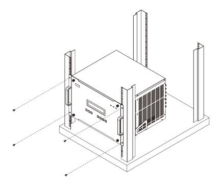
**Note:** To ensure the VW3620 has sufficient air flow, do not stack items around the unit. Proper air flow ensures safe operation and prevents the unit from overheating.
