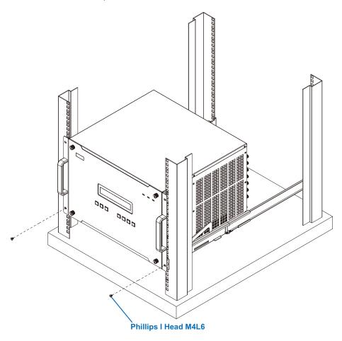
**Note:** To ensure the VW3620 has sufficient air flow, do not stack items around the unit. Proper air flow ensures safe operation and prevents the unit from overheating.
