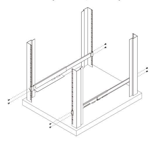
2. Push in and lock the recessed handles, and then slide the unit along the brackets.
