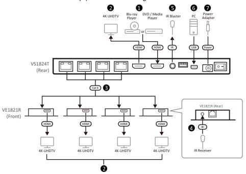
**Note:** A VS1824T splitter is used as an example to illustrate the installation. As for VS1828T splitter, it is equipped with 8 link ports for connecting up to 8 VE1821R receivers.
