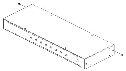
2. Use the M3 x 8 Phillips head hex screws supplied with the rack mounting kit to screw the rack mounting brackets into the rear of the unit.
