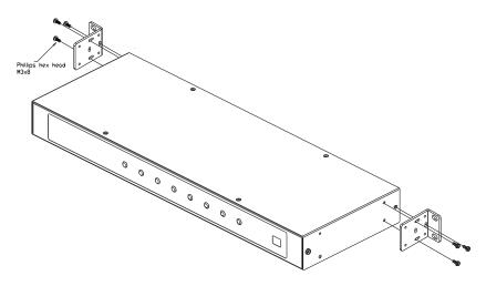
3. Position the device in the rack and align the holes in the mounting brackets with the holes in the rack.
