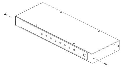
2. Use the M3 x 8 Phillips head hex screws supplied with the rack mount kit to screw the rack mounting brackets into the front of the unit.
