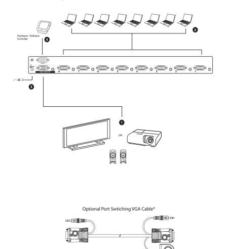
\*The optional *Port Switching VGA Cable* shown above provides a high quality VGA cable with port switching button to switch the VS0801A to the source device it is connected to when pressed. This optional accessory is installed between the VS0801A and a source device, as shown in step 2. The *Port Switching VGA Cable* can be purchased separately from your local ATEN dealer.
