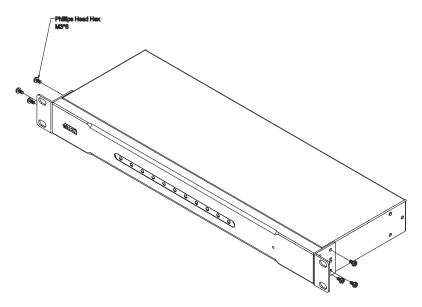
2. Screw the mounting brackets to the rack.
