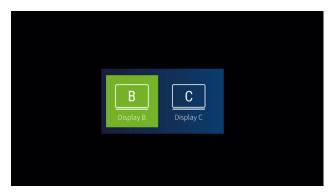
4. Navigate to the display you wish to control and then press the **Enter** button/pushbutton. You can now use the OSD to remotely control the display. The OSD changes to red and the controlled display is indicated.
