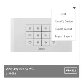
b) From the pop-up web page, configure the Remote Pad's layout. For details about the configuration fields, refer to the ATEN Remote Pad User Manual.
