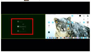
c) Use the Up and Down buttons/pushbuttons to select a source. The selected source is immediately applied.
