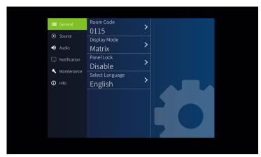
4. Navigate to **General > Display Mode** and then select a view mode. The view mode is immediately applied to the connected displays.
