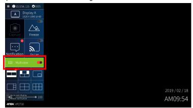
To change the multiview layout navigate to a layout you wish to use and press the Enter button/pushbutton. The layout is immediately switched.
