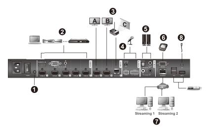
1. Use a grounding wire to ground the unit by connecting one end to the grounding terminal, and the other end to a suitable grounded object.
