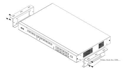
Position the unit to a spot under the desk where you can easily access the front-panel pushbuttons, and then secure the racks to the desk with selfprepared screws.
