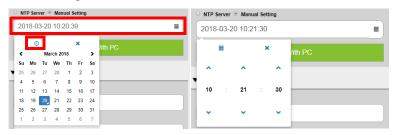
• Sync with PC: Click this button to synchronize the VP2730's date and time with the PC with which the web interface is opened.
