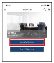
5. Enter the IP address of the VP2730 and room code (see *System Settings*, page 29 for details), and then tap **Connect**.
