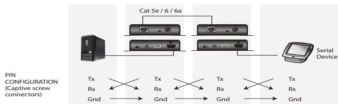
From a source device, the RS-232 signal is transmitted (Tx) to the VE3912T receiving (Rx) unit; the a compatible ATEN Video Receiver transmits (Tx) signals to the display device (Rx).
