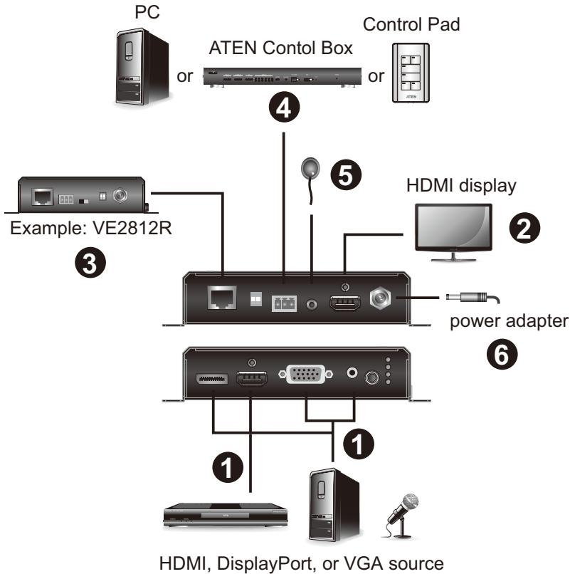
1. Connect the DisplayPort, HDMI, and/or VGA input port on the VE3912T to the DisplayPort, HDMI, and/or VGA sources using the required cables respectively. If VGA is connected, then you need to connect the VGA audio jack to the audio input on the VE3912T to transmit sound.
