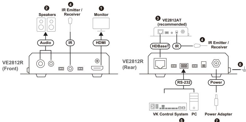
1. Connect an HDMI-enabled display to the VE2812R's HDMI out port.
