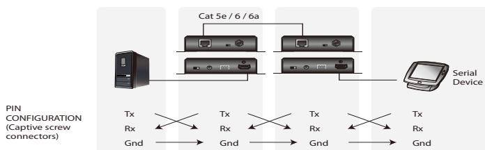
From a source device, the RS-232 signal is transmitted (Tx) to the VE2812R / VE2812PR receiving (Rx) unit; the a compatible ATEN Video Receiver transmits (Tx) signals to the display device (Rx).
