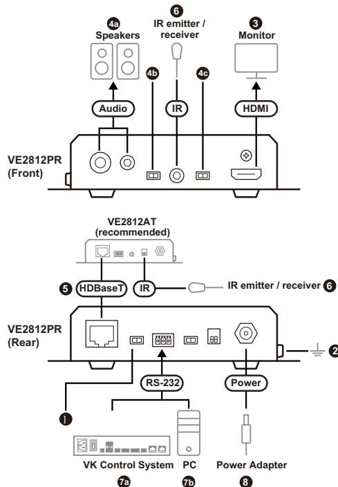
1. Before installation, please make sure the VE2812PR is set to PoH PSE or PoH PD mode using the DIP switch for your installation requirement.
