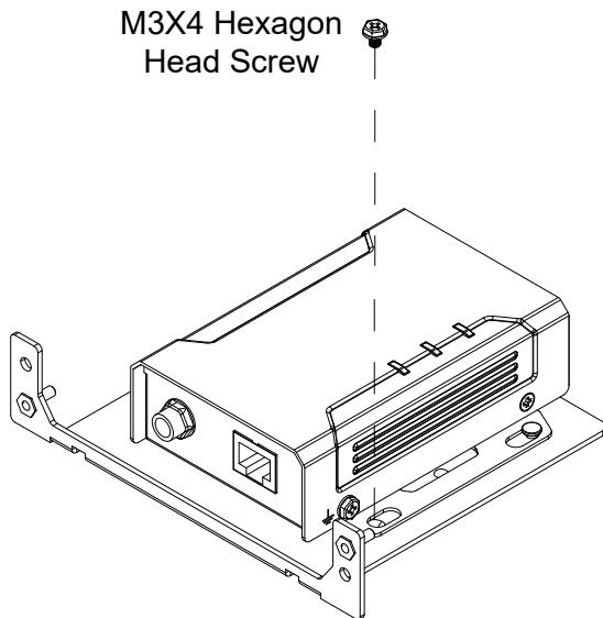
4. If the video extender doesn't have a mounting bracket, align the bottom holes and then screw the video extender to the mounting plate.
