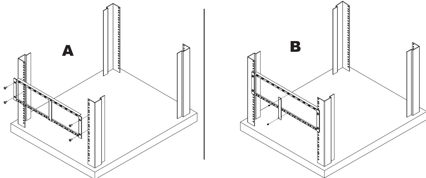
2. Place the Video Extender over the 3U Mounting Plate and bring the two pieces together so that the mounting post enters the rear hole. Next, slide the Video Extender forward to lock it in place. For video extenders without brackets, see step 4.
