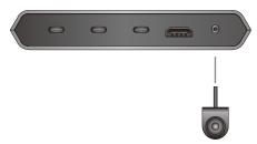
2. Prepare a USB Type-A to Type-C cable. Connect one end of the USB Type-A cable to the computer and the other end to the US3310 USB 3.2 Gen 1 Type-C Port 1.
