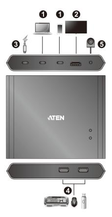
1. Plug the USB Type-C cable between your computer and/or mobile device into the back of the US3310.
