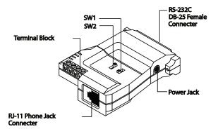
The IC-485SN is configured by setting two slide switches. SW1 is used to select the *Device Mode*; SW2 is used to select the *Transmitting and Receiving Mode*, as shown in the table below:
