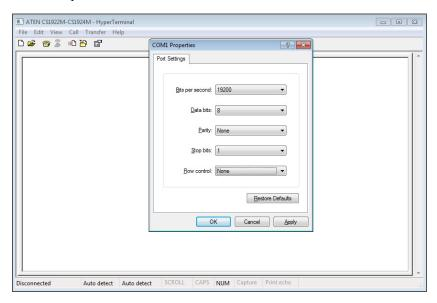
Bits per Second: **19200**, Data Bits: **8**, Parity: **None**, Stop bits: **1**, Flow Control: **None**.
