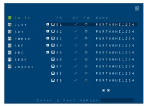
Clicking [f] G O T O or pressing [F1] activates the Go To function. Go To allows you to switch directly to a port by keying in the port's ID. Enable mouse emulation for independent switching (see page 42), for this function to work.
