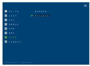
Clicking SCAN or pressing [F7] invokes *Auto Scan* mode. This function allows you to automatically switch among the available computers at regular intervals so that you can monitor their activity without having to take the trouble of switching yourself. Enable mouse emulation for Auto Scan to work (see page 42).
