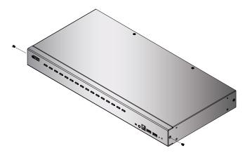
2. Use the M3 x 6 Phillips hex head screws supplied with the rack mounting kit to screw the rack mounting brackets into the sides near the front of the unit.
