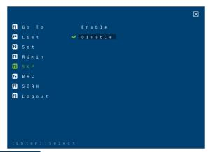
Clicking S K P or pressing [F5] invokes Skip (SKP) mode. This function enables you to easily skip backward or forward – switching the console focus from the currently active computer port to the previous or next accessible one. Enable mouse emulation for Skip mode to work (see page 42).
