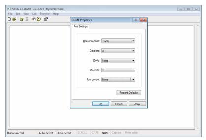
Bits per Second: **19200**, Data Bits: **8**, Parity: **None**, Stop bits: **1**, Flow Control: **None**.
