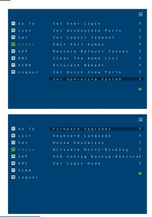
Clicking Admin or pressing [F4] activates Admin function. F4 is an administrator only function. It allows the administrator to configure and control the overall operation of the OSD. To change a setting, click on the settings item you want to configure, or use the up and down arrow keys to move the highlight bar to it then press [Enter].
