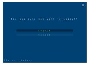
Clicking Logout, or pressing [F8] logs you out of OSD control of the computers, and blanks the console screen. This is different from simply pressing [Esc] when you are at the main screen to deactivate the OSD. With this function you must log in all over again to regain access to the OSD, whereas with [Esc], all you have to do to reenter the OSD is tap the OSD hotkey.
