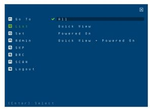
Clicking List or pressing [F2] activates the List function. This function lets you broaden or narrow the scope of which ports the OSD displays on the main screen. The submenu choices and their meanings are given in the table below.
