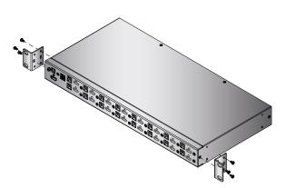
3. Place the KVM switch in the rack. Position it so that the holes in the mounting brackets line up with the holes in the rack. Secure the mounting brackets to the rear of the rack.
