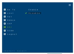
F6 is an administrator only function. Clicking BRC or pressing [F6], invokes *Broadcast* (BRC) mode. When this function is in effect, commands sent from the console are broadcast to all available computers on the installation.
