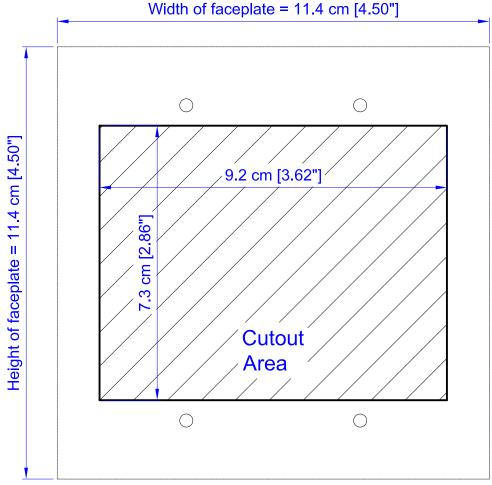
**Note:** ATEN recommends a 2-gang wall box with a depth of at least 4.5 cm (1.77 inches) to accommodate the connectors and cables.
