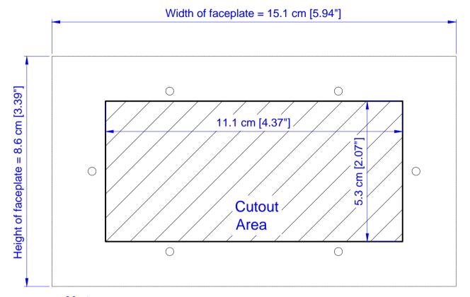
**Note:** ATEN recommends a 1-gang wall box with a depth of at least 3.6 cm (1.42 inches) to accommodate the connectors and cables.
