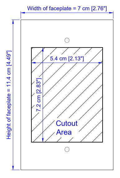
Note: ATEN recommends a 1-gang wall box with a depth of at least 6 cm (2.36 inches) to accommodate the connectors and cables.
