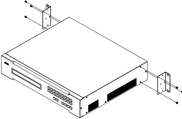
2. Position the unit in the front of the rack and align the holes in the rack mount brackets with the holes in the rack.
