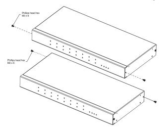
2. Screw the mounting brackets into the sides of the unit at the front or the rear, as shown in the diagram below.
