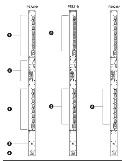
**Note:** The PE7216r / PE8216r / PE9216r unit components are identical except for the outlet LEDs – the PE7216r has none; the PE8216r has 16; and the PE9216r has 8, as shown by number 9 above.
