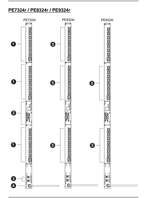
**Note:** The PE7324r / PE8324r / PE9324r unit components are identical except for the outlet LEDs – the PE7324r has none; the PE8324r has 16; and the PE9324r has 8, as shown by number 5 above.
