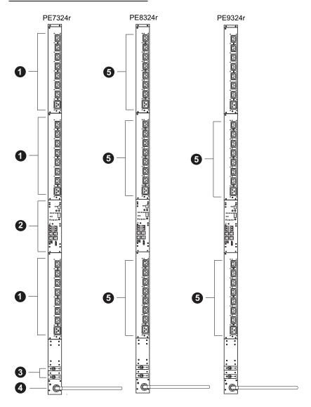
**Note:** The PE7324r / PE8324r / PE9324r unit components are identical except for the outlet LEDs – the PE7324r has none; the PE8324r has 16; and the PE9324r has 8, as shown by number 5 above.
