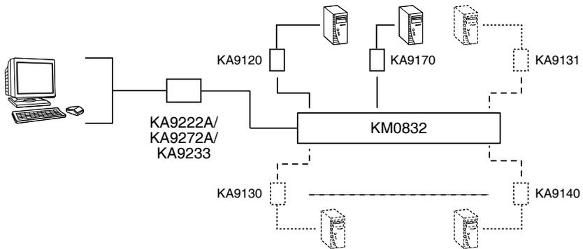
A separate console module is required for each KVM console; likewise, a separate KVM adapter cable is required for each computer. The console modules and KVM adapter cables are listed in the *Cables* section on page 5. Consult your dealer to find out which console modules and KVM adapter cables best fit your needs.
