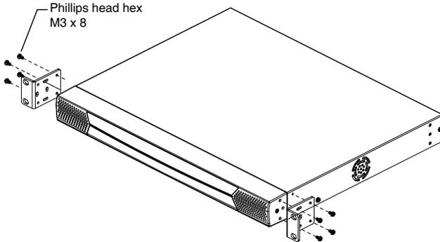
3. Place the KVM switch in the rack. Position it so that the holes in the mounting brackets line up with those in the rack. Secure the mounting brackets to the front of the rack.
