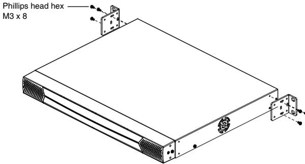
3. Place the KVM switch in the rack. Position it so that the holes in the mounting brackets line up with those in the rack. Secure the mounting brackets to the rear of the rack.
