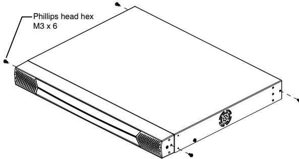
2. Detach the front panel from the chassis; however, leave the cables attached. Use the M3 x 8 Phillips head hex screws supplied with the rack mounting kit to screw the rack mounting brackets into the sides of the front panel and chassis.
