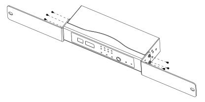
2. Position the unit in the front of the rack and align the holes in the mounting brackets with the holes in the rack.
