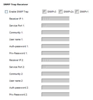
Up to four SNMP management stations can be specified. If you want to use SNMP trap notifications, do the following:
