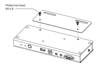
2. Screw the bracket into any convenient location on the rack.
