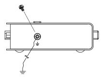
2. Make sure that the computer that the CE800BL connects to and the monitor that the CE800BR connects to are properly grounded.
