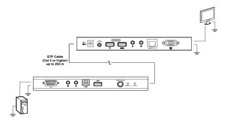
3. See the Grounding Information card that came with this package for proper grounding details.
