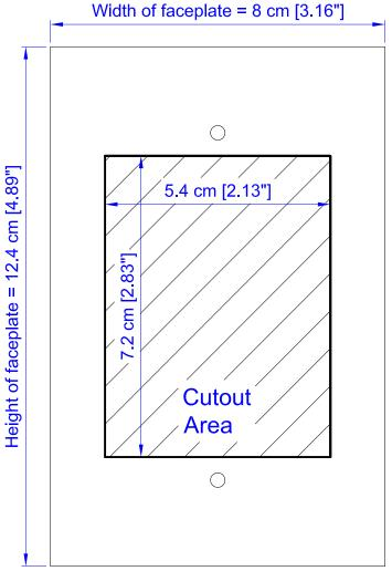
Note: ATEN recommends a 1-gang wall box with a depth of at least 5 cm (1.97 inches) to accommodate the connectors and cables.
